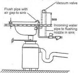
This figure shows the installation of a vacuum valve above a sink assembly. In your case the assembly used may be of another type (not a sink). The positioning of the vacuum valve is however the same.
