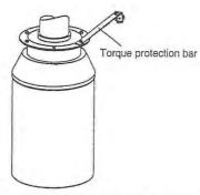
If a torque protection bar is not suitable because the distance to the wall / bulkhead is too far, torque protection clamps can be fixed around the disperator legs to the floor / floor plate instead as per the figure below.
